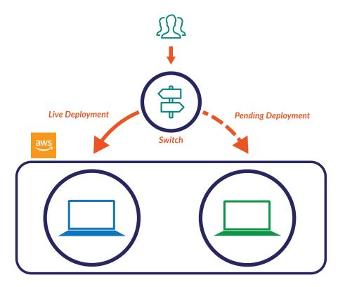
With Blue/Green deployment, the current RTSM (blue) is cloned to RTSM (green). The upgrades are performed on the cloned RTSM Green. This way, if anything were to go wrong during the upgrade itself, the original RTSM Blue is left untouched. Upgrades can be done in as little as 10 minutes up to 1 hour depending on the scope of the upgrade. Upgrades are scheduled ahead of time to ensure no disruption to a study (e.g. midnight on a Saturday).
